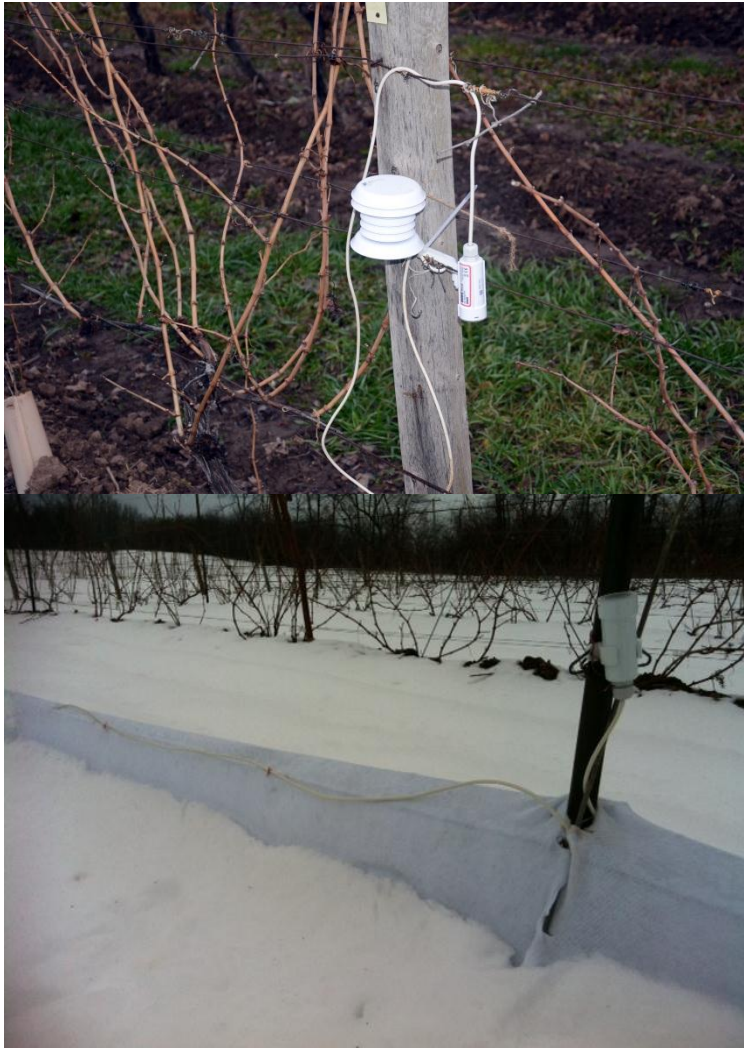
Image 4. Data loggers used to monitor impact of geotextiles on vine microclimate
