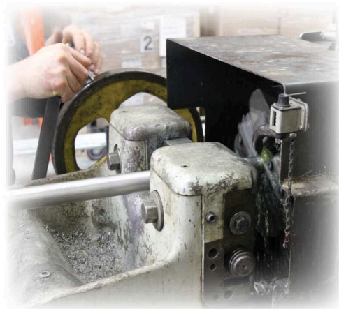
Threading of 304SS stand pipe for the YHSS Series hydrants
