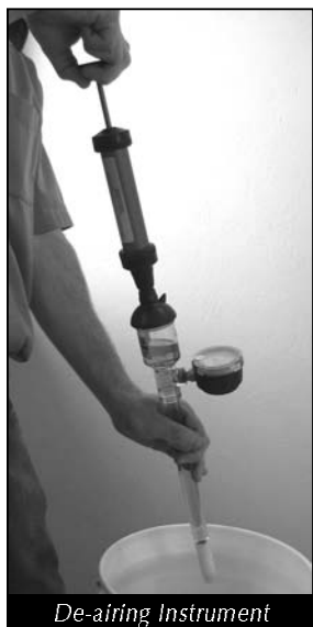
De-airing in the Ground
