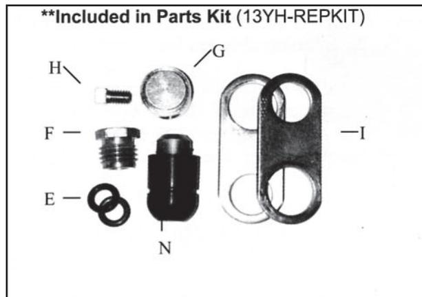
**NOTE:** In the event that the plunger (N) needs changing, loosen set screw (H), place wrench on the hydrant head (A) and unscrew. Place vise-grips on connecting rod (P) and pull rod and plunger out of valve body. Replace with new plunger and re-assemble unit. Re-set operating rod and tighten set screw.
